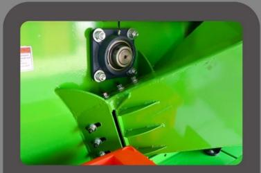
Traditionally, wood chippers rely on a single anvil to smash branches against the spinning blades. But the Yardbeast 6525 doubles down with two strategically positioned anvils that corners the branch up at the top, creating an amazing self feeding effect on a wide array of woods and fibrous material like palm fronds.
