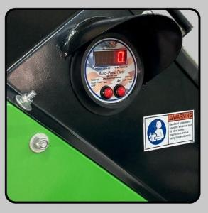
Electronic programmable hydraulic feed controller allows the chipper to maintain optimal blade RPM when chipping. Reverse and delay programmable.
