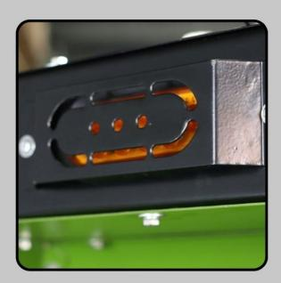
Auto warning light that turns on automatically when the engine is started alerting operators and bystanders that the chipper is currently under power.
