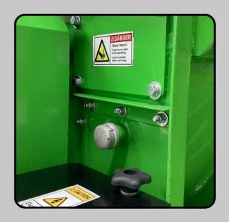
Blade change port allows quick inspection or change of the edge of the blade, or perform a blade replacement. Safety is improved with rotor locking mechanism.
