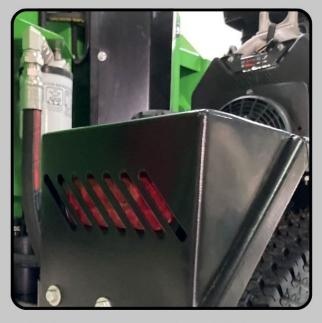
DOT compliant enclosed lightning on the trailer with standard 4prong connector terminal and 2inch side turn signals.
