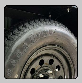
ST235/85-15 high speed tires coupled to a torsion axle-less suspension for a smooth highway and offroad ride and superior overcome of obstacles.
