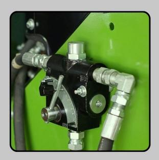
Cast-iron heavy duty Hydraulic fluid regulator controls the feeding speed of the feed roller. A 1,500 psi preset safety valve ensures system safety at maximum loads.
