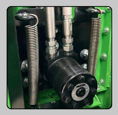
Feeding assembly comprises of a single 10-inch feed roller controlled by four tension springs. Carriage is mounted on 8-angular sealed bearings for superior responsive feeding. Hydraulic motor delivers up to 2,150 lb-in torque at slow speeds. Feeding speed up to 200 ft/min. Feeding system is completely enclosed to increase operator safety.
