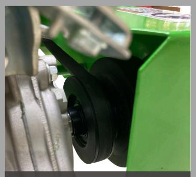
The engine is fitted with a Hilliard® heavy duty centrifugal clutch that engages or disengages when the engine reaches 1,800RPM. A clutch allows user to start the engine easily.
