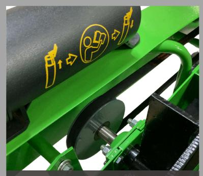
This transmission system features a single pulley with a tapered hub. This design minimizes wobbling and ensures smooth transmission of rotational force (torque).
