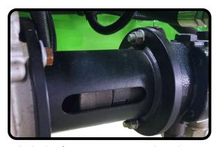
The hydraulic pump is connected to a heavyduty flexible coupler that makes the engine and pump run smoothly.
