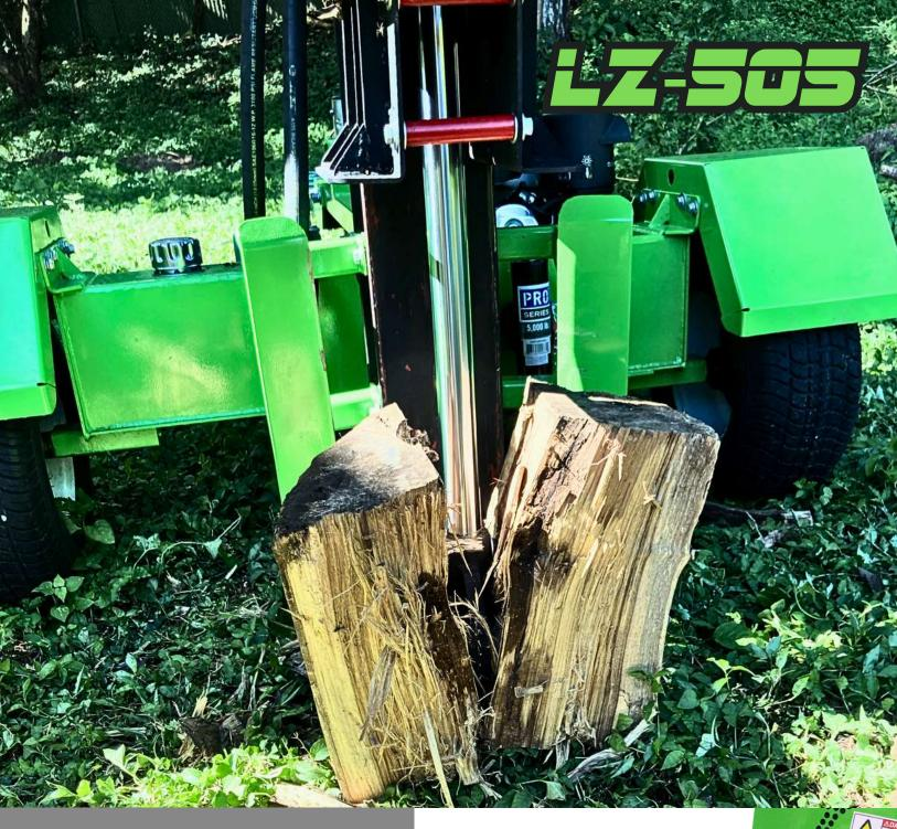
The splitter wedge is machined with a razor sharp edge and welded with split flaps to allow quick wood detachment. The splitter wedge can be switched to a 4-way splitter if needed. All splitting wedges are heat treated for improved abrasion resistance.
