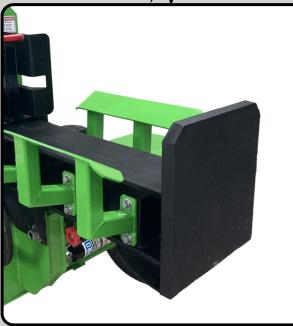
The boot of the beam is fabricated from 1" thick steel, allowing the splitting wedge to demolish even the toughest knots! The design includes removable trays for versatility, allowing you to attach various accessories like extended log handling trays for your needs.
