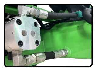
The dual-stage pump delivers up to 22 GPM. The first stage fills the hydraulic cylinder quickly, and the second stage kicks in at the log splitting moment to achieve peak split force.
