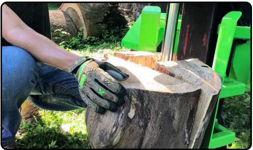
The Yardbeast LZ-505 is designed with ergonomics in mind to make log splitting more efficient and comfortable. The splitting cradle is positioned at a user-friendly height of 32 inches off the ground, allowing for accurate placement and control when handling heavy logs. The controls are conveniently located on both sides of the tray, accessible whether you're using the splitter in its horizontal or vertical mode.
