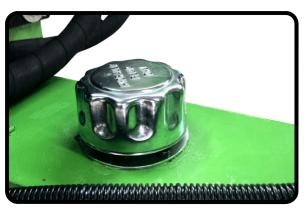
Deluxe accessories on the splitter are standard, like a hydraulic oil cap with strainer. and internal magnetic debris plug. All trailer light connections are enclosed in DOT approved loom cable.
