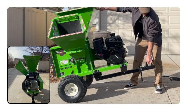
The Yardbeast 2090 lets you switch between a hitch pin or ball trailer coupler (optional) for effortless movement around your property with your ATV vehicle or truck. Plus, the wide 16-inch wheels ensure a smooth ride and help you avoid bumps and obstacles. And the best part? The fully bolted trailer tongue makes it highly adaptable. Need to connect the chipper to a different towing setup for a specific job? No problem! Also available a tongue wheel dolly if you need to tow it by hand.
