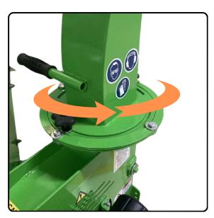
You can choose where to throw the chips by rotating the discharge chute. SImply loosen two knobs and move where desired. To adjust throwing distance, you can adjust chip deflector.
