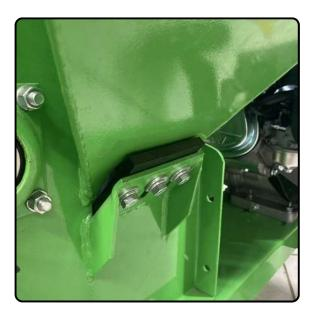
3/8 inch thick adjustable anvil with dual edge, can be flipped over to extend resharpening intervals. Anvil base is double welded all around to significantly increase its load support.
