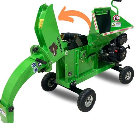
Say goodbye to complicated maintenance! The Yardbeast 3514 boasts a simple yet effective splitchipper frame design. Simply lift the top cover and the entire chipper frame hinges open, exposing the chipper rotor in all its glory. This unique approach grants you unprecedented access for routine maintenance. Replacing the blade, cleaning internal components, and adjusting the anvil-blade gap become effortless tasks.
