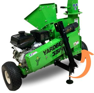
Your Yardbeast 3514 ATV hitch can easily be transformed from a pin hitch to a ball coupler style giving you the ability to tow this chipper with different vehicles.
