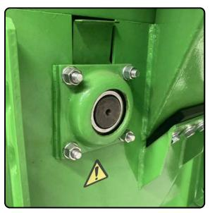
Bearing units come with metallic seal that protects the inner tracks and balls, extending the operational life of the units making them virtually maintenance free.
