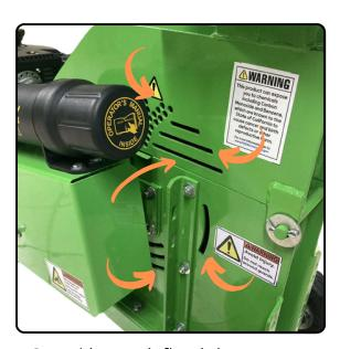
On a chipper, air flow is important to cool components, while carrying wood chips out of the chipper and discharge them as far as possible. Uniquely designed hole pattern optimizes air flow through the 3514 while keeping the chipper cool.
