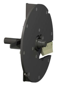
The rotor is a wafer-type design with a overall 7/16" thickness. The design is a single blade rotor that is dynamically balanced. This configuration allows the Yardbeast to deliver an unprecedented performance since it allows the chipper o recoup inertia and engine speed a full turn for every cut! The rotor comes with 4 vanes in the back that creates airflow while throwing
