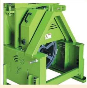
The PTO driveshaft is rated for CATO-1 tractor for 540RPM input up to 45HP. The drive is composed of a 1:3 pulley transmission with 3-type V belts spinning the rotor up to 2,300RPM.
